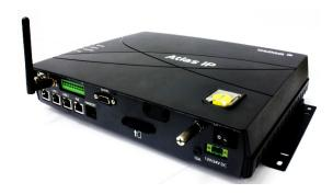
The BDU has a built-in Web Console, which can be accessed from a computer connected to the BDU, using an Internet browser. The Web Console provides easy configuration of the BDU, firmware upgrade and daily use. For more information, refer to the chapter of the Web Console.
