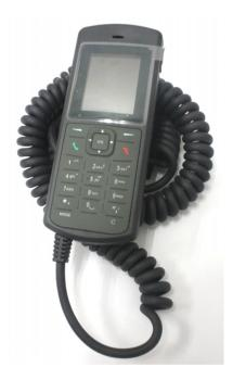
The wired Primary Handset has a colour LCD and keypad for making and receiving voice calls and sending SMS using an interface similar with a mobile phone. It can serve as a remote access for user to access various BDU functions. The Primary Handset connector is plugged into the BDU primary handset port and it is powered directly from the BDU.
